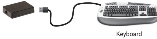
FIGURE QS-3. CONNECT THE USB DEVICE(S) TO THE REMOTE EXTENDER
