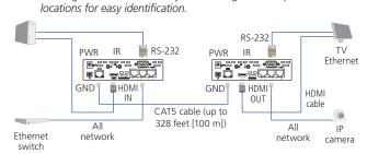
CAUTION: The CAT5e/6 cables that connect the Transmitter and Receiver Units carry electrical current and should not be plugged into other devices, because they may cause damage to them. We strongly recommend marking the CAT5e/6 cables you are using with this product at both
