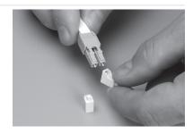
STEP 2: Hold the fiber assembly with the pull tab down. With your left hand, hold the assembly housing and with your right hand, pull the boot away.
