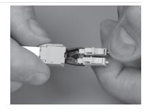
STEP 6: Finally, slide the boot up to the housing back in its original position covering the silver crimp ferrule.
