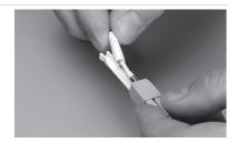
STEP 3: Using a small flat screwdriver, place the tip under the rear latch of the assembly housing. Slightly twist the screwdriver to release the housing while pulling back exposing the black inner body.
