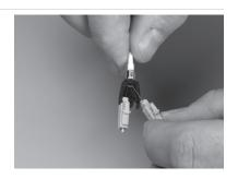
STEP 5: Next, with your left hand, hold and press on the locking tab of the two LC connectors. With your right hand, slide up the assembly housing back into its original position.
