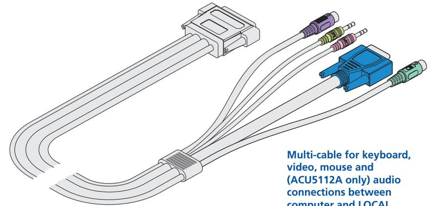
**Multi-cable for keyboard, video, mouse and (ACU5112A only) audio connections between computer and LOCAL module**
