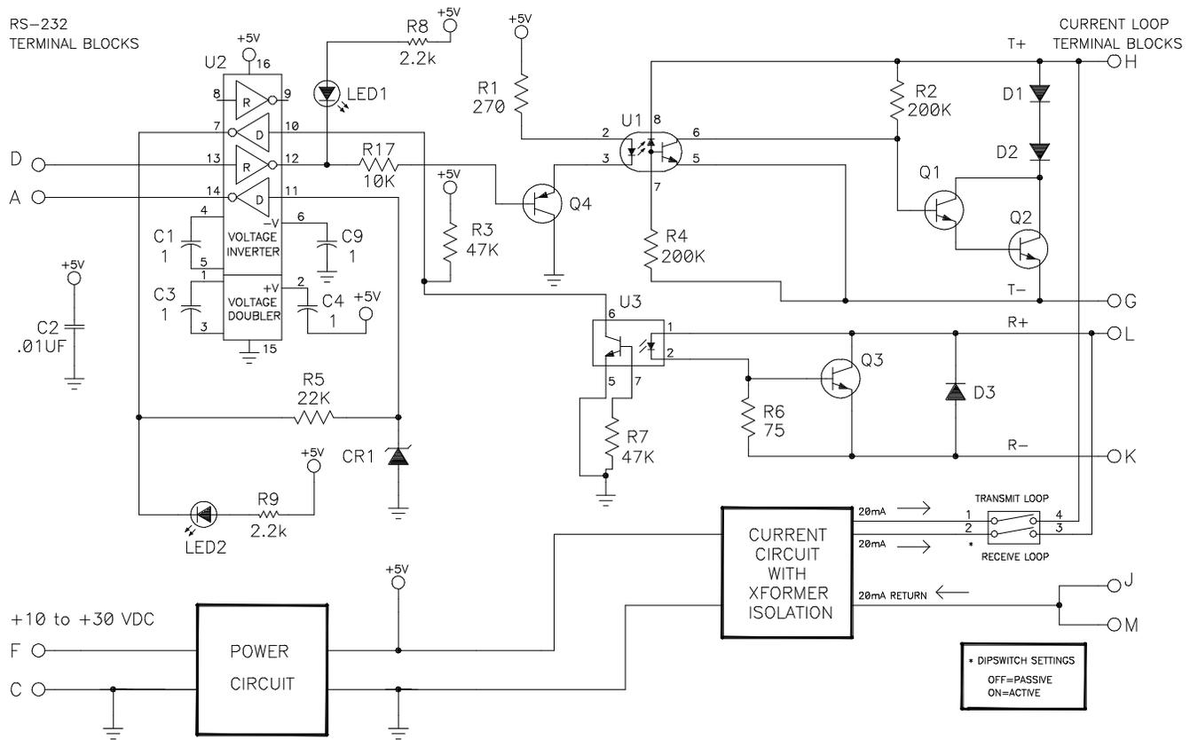
Figure 7. ICD101A Schematic
