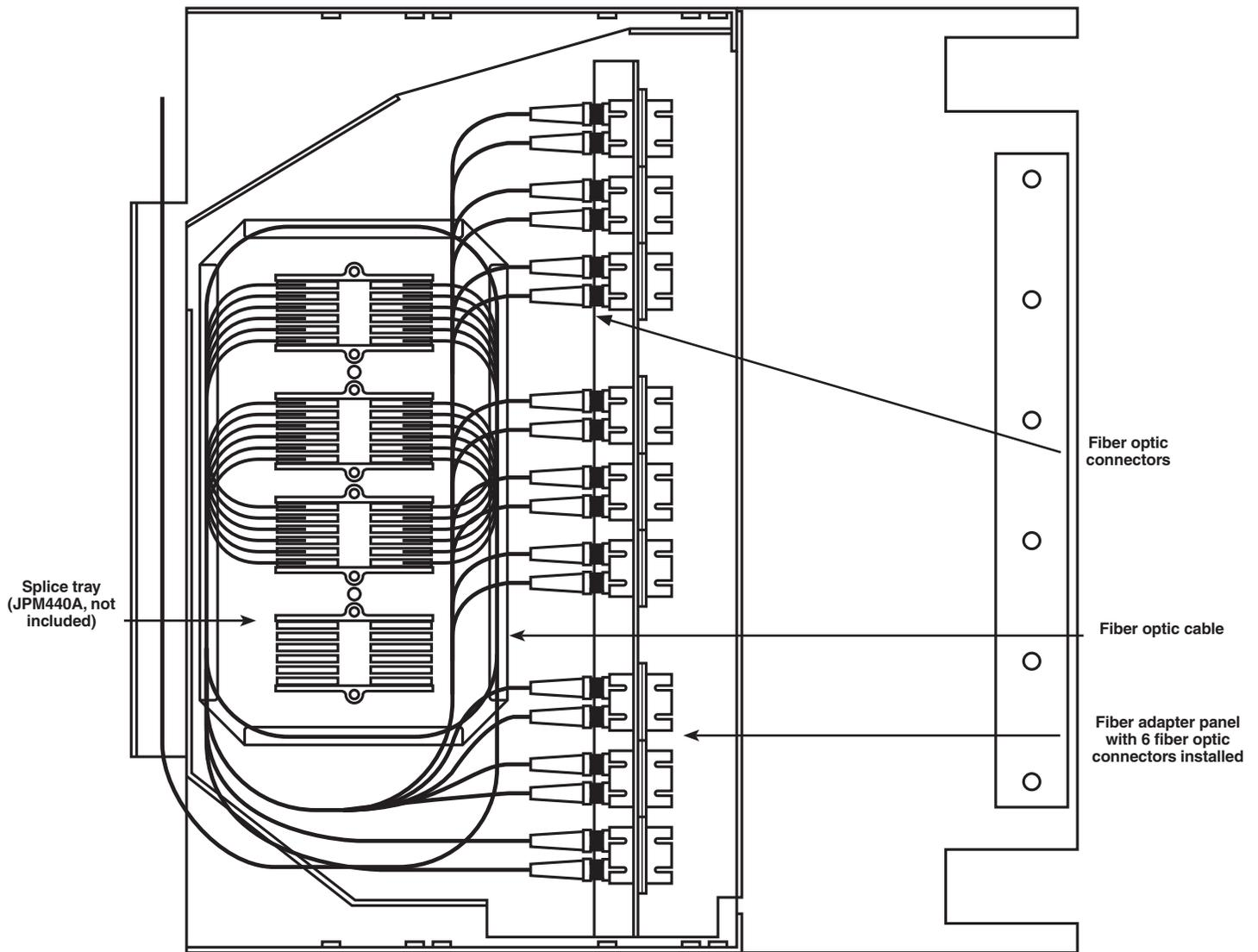
**Figure 2. The JPM406A-R5 with three fiber adapter panels visible (up to nine more can be stacked beneath the visible ones, for a total of 12 adapter panels). The fiber cable is routed through the splice tray, then terminated via the fiber optic connectors.**
