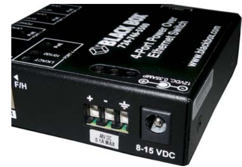
Figure 2.1b. BlackBox LP004A. Rear view (one RJ-45 port (not shown) and DC terminal and power adaptor option on rear side) as shown in Fig 2.1b.
